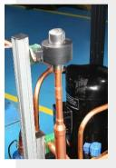
With electronically controlled capacity regulating valve (Selected capacity only), Summits Refrigeration air dryer keeps the Pressure dewpoint nearly constant even in wide operating range with quantum jump load variation.
